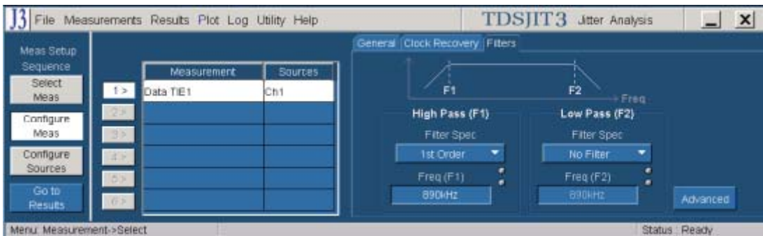
Figure 97: Configuring filters for a 1.5 Gbps SAS device
