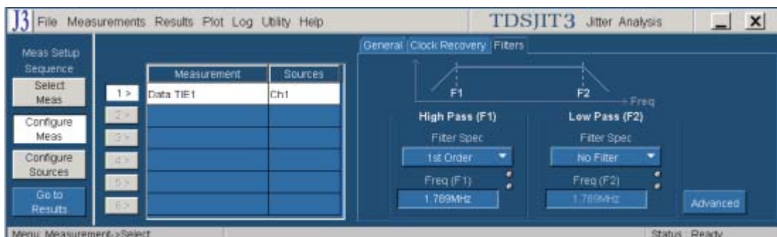
Figure 98: Configuring filters for a 1.5 Gbps SAS device
